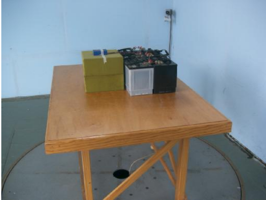
Photo 1. Electromagnetic Radiated Emission Test Configuration.
