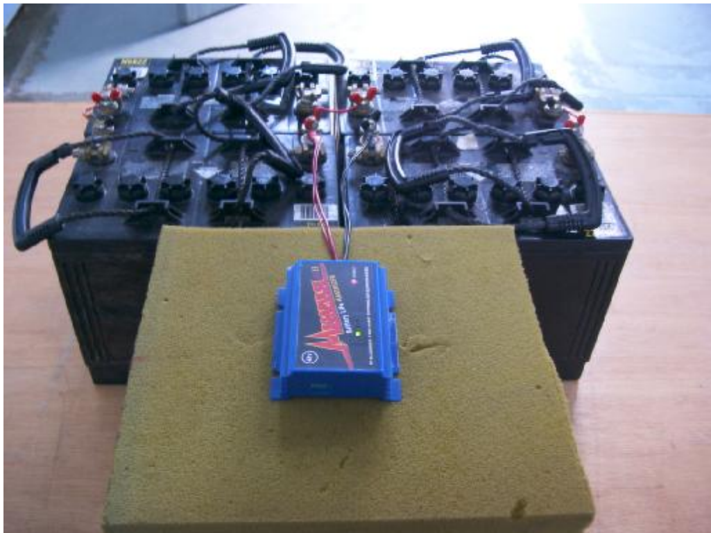
Photo 2. Electromagnetic Radiated Emission Test Configuration Close Up.
