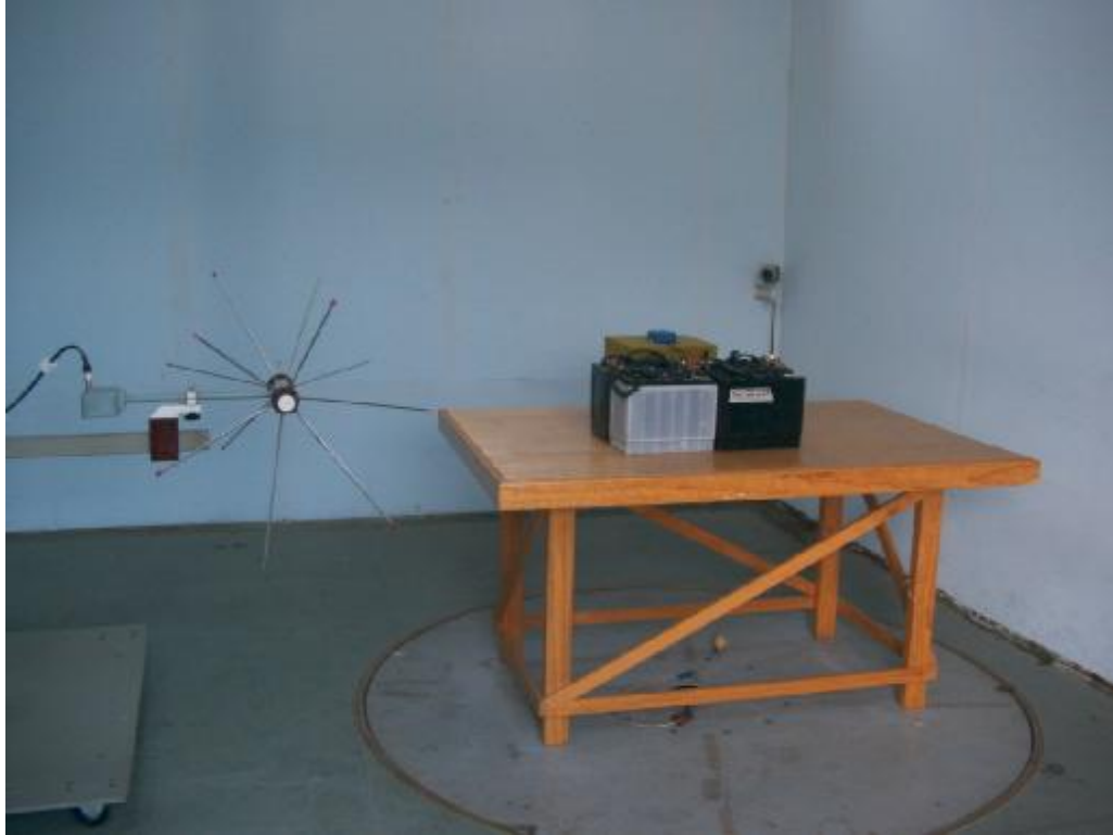
Photo 1. Electromagnetic Radiated Emission Test Configuration.
